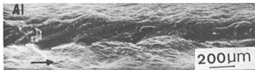
Figure 9 Increasing apparent striation spacing in Al with increasing crack length. The arrow indicates the crack growth direction.
